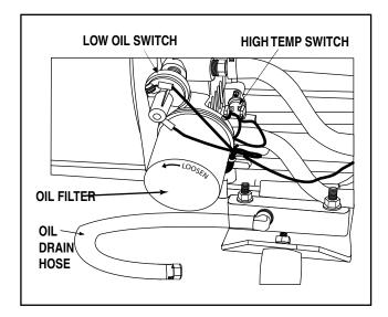
Figure 1. Engine Protective Switches on an Air-Cooled Engine
